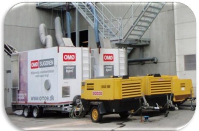
OMØ Mobile Fan is mounted on a trailer so that it can be used almost anywhere.
